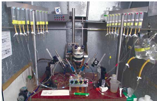
Left: A patch-clamping rig set up to record the flow of ions through receptor channels in the large immature egg cell (oocyte) of the frog Xenopus .
