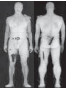
Backscattered x-rays aren't used on airline passengers in the United States (most people would object to an instrument that can essentially strip them naked), but they can illuminate hidden weapons very clearly, as the man above demonstrates—a metal gun and a scalpel blade in the front view and a metal file, plastic knife and plastic gun (a Glock 17) in the back. Backscattered x-rays can also pick out illegal aliens being smuggled in a truckful of bananas (right). (Images on this page courtesy of American Science and Engineering.)
