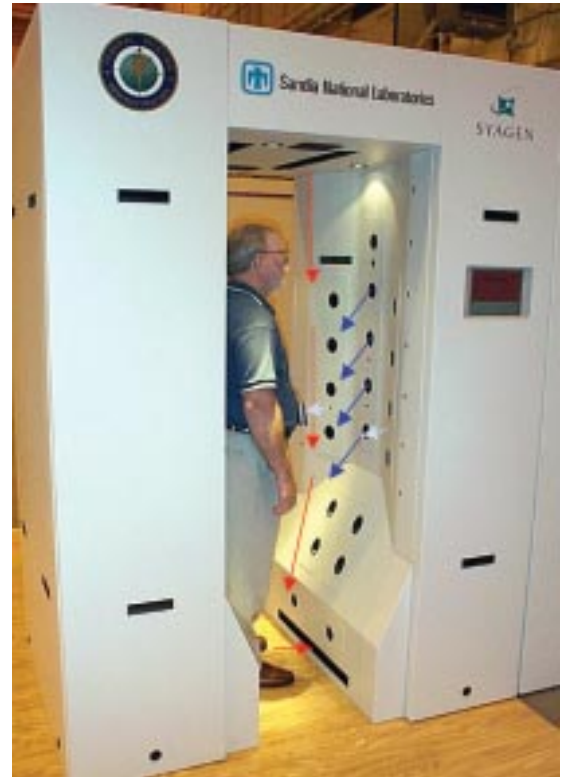
Above: In the Syagen portal, the main stream of air flows past the subject (red arrows), as pulses of air (blue arrows) puff his clothing to liberate particles, while other jets of ionized air help collect them (white arrows). Next the particles pass into a time-of-flight mass spectrometer (opposite page), which delivers the mass spectrometric fingerprints for several common explosives (below). (Illustrations courtesy of Syagen Technology, Inc.)
