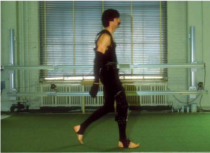
Above: Antonsson makes great strides toward his PhD. The round things strapped to his body are plates bearing LEDs, whose travels are recorded by the two infrared cameras on the adjustable rails in the background. (In a real experiment, the LEDs would be facing the cameras.)
