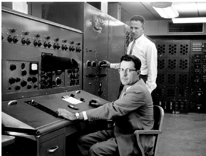
McCann sits at the console of his direct analogy electrical analog computer, a behemoth that took up all sides of this large room in 1958. The results of engineering calculations were read from the oscilloscope above the console.
