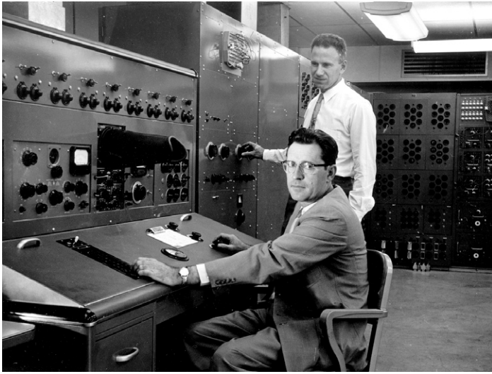
McCann sits at the console of his direct analogy electrical analog computer, a behemoth that took up all sides of this large room in 1958. The results of engineering calculations were read from the oscilloscope above the console.
