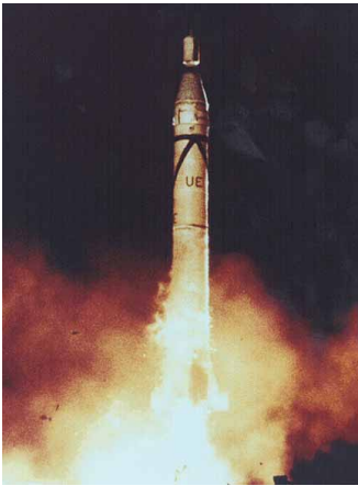
Explorer 1 lifted off at 10:48 p.m. on January 31, 1958, on a Jupiter-C rocket, von Braun’s modification of the Redstone ballistic missile that was itself a direct descendant of the German V-2. The Army Ballistic Missile Agency and JPL finished modifying the rocket and built and launched Explorer in just 84 days.
