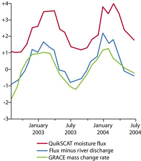
**Above: Space-based measurements of the moisture flux over South America (red line) are tracked from space by the Quick Scatterometer. From these measurements is subtracted the water loss from the continent measured with ground-based river gauges. The resulting water balance (blue line) matches both in amplitude and phase the mass changes (green line) measured from space by the Gravity Recovery and Climate Experiment (GRACE).**
