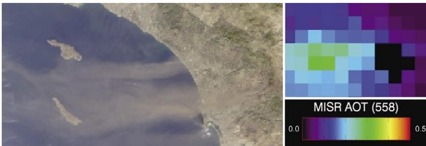
**As opposed to ash in the upper atmosphere, dust in the lower atmosphere absorbs sunlight and can warm the atmosphere. These dust clouds off of Southern California are mapped using the optical depth determinations of the MISR instrument.**
