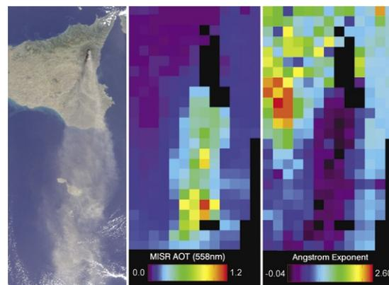
Ash erupted from volcanoes can significantly cool the planet by blocking sunlight from reaching Earth's surface. MISR images from the 2002 eruption of Mount Etna helped determine the aerosol optical thickness (AOT, middle panel), or how difficult it is to see through the ash plume. In the Angstrom exponent map (right panel), which shows the distribution of particle size, the ash plume is easily discerned.
