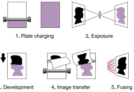
**How xerography works:** A specially prepared plate is charged with static electricity (purple). The charge drains away wherever light hits the plate; dark areas remain charged. A black powder of opposite charge will stick only to those areas, and when a piece of paper is pressed against the plate the powder (and the image) is transferred. Heat treatment binds the powder to the paper.
