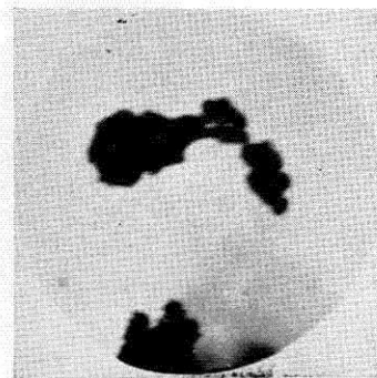
Fig. 2: A shot of Optical Rouge taken with the instrument of Fig. 1 Magnification: 16,500 diameters.
