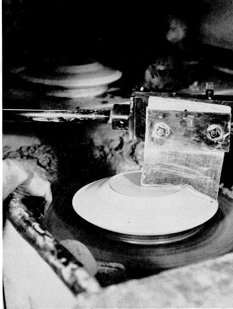
Flat ware is produced by the jigger method, a modification of the potter's wheel.
