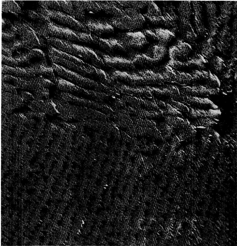
FIG. 4—Pearlite in steel. A lamellar arrangement of iron and brittle iron carbide. The magnification is 20,000 diameters.
