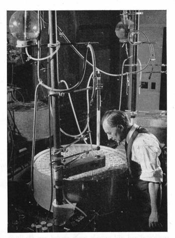
BIOLOGY: Electronically controlled machine built by Dr. Henry Borsook (above) and Dr. Geoffrey Keighly helps Caltech biochemists separate and collect proteins and amino acids — the fabric of all living cells.
